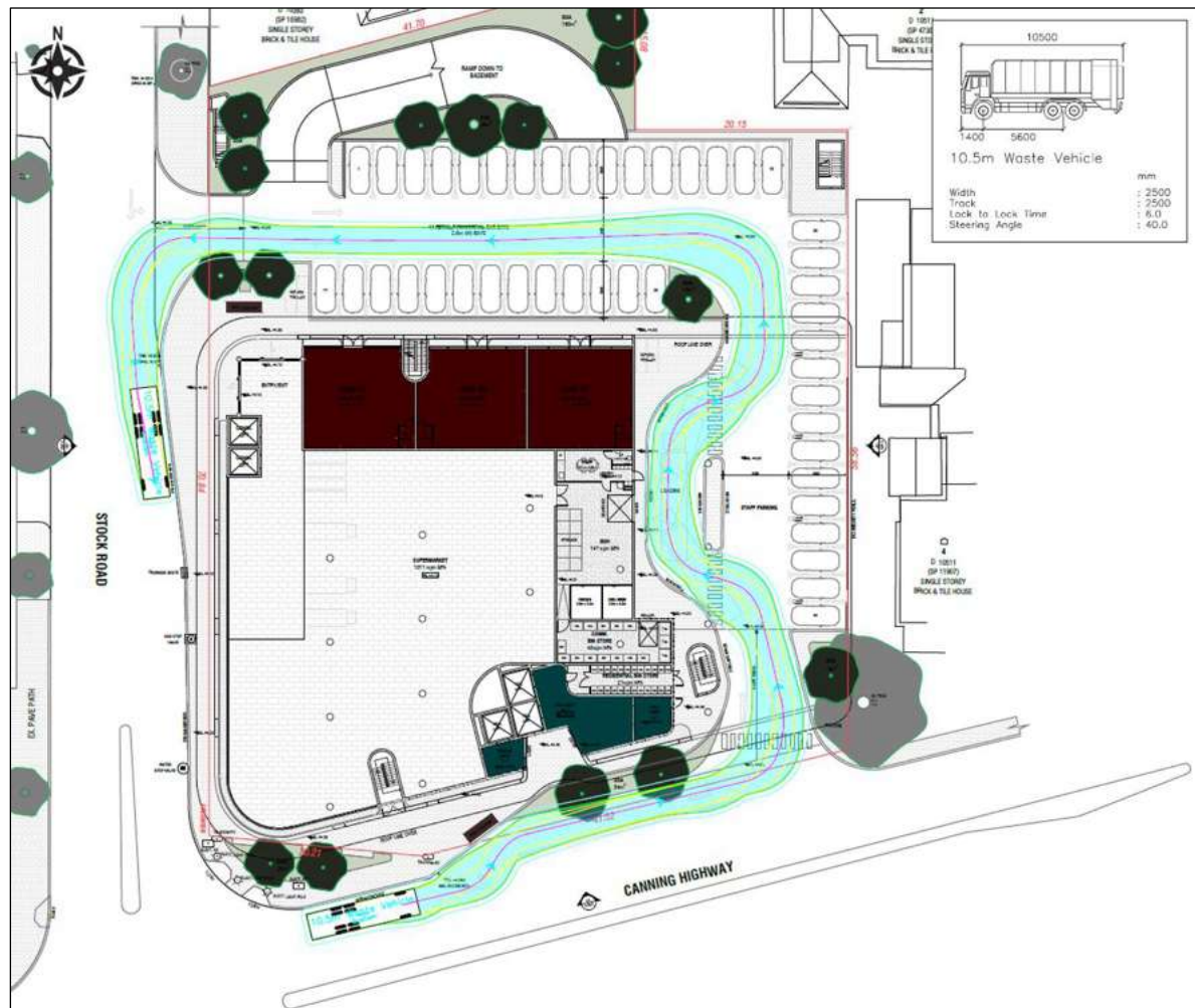
Figure 8 Swept Path - Waste Truck
